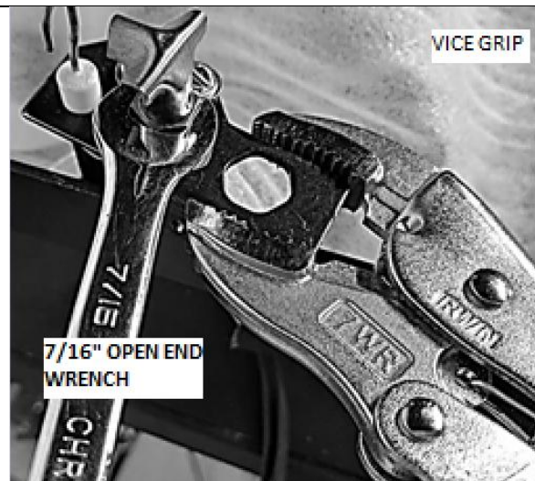
Figure 4-6 Pinch Pilot Base with Vice Grips
