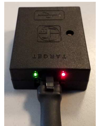
Fig.3: WiFi dongle connected to the IFC
